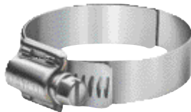
Series 92208 through 92248 For Use on Silicone Hose Silicone clamps with extended inner liner covering band slots to prevent hose damage featuring zinc dichromate plated slotted hex head screws
